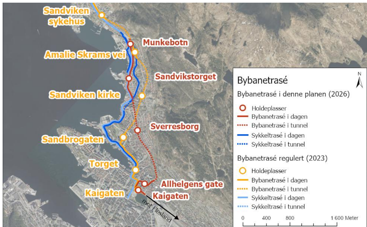
Figure 1-4: Comparison of the Bergen Light Rail (Bybanen) alignment and stop locations between the approved zoning plan currently in force (orange) and the proposed plan (red).
