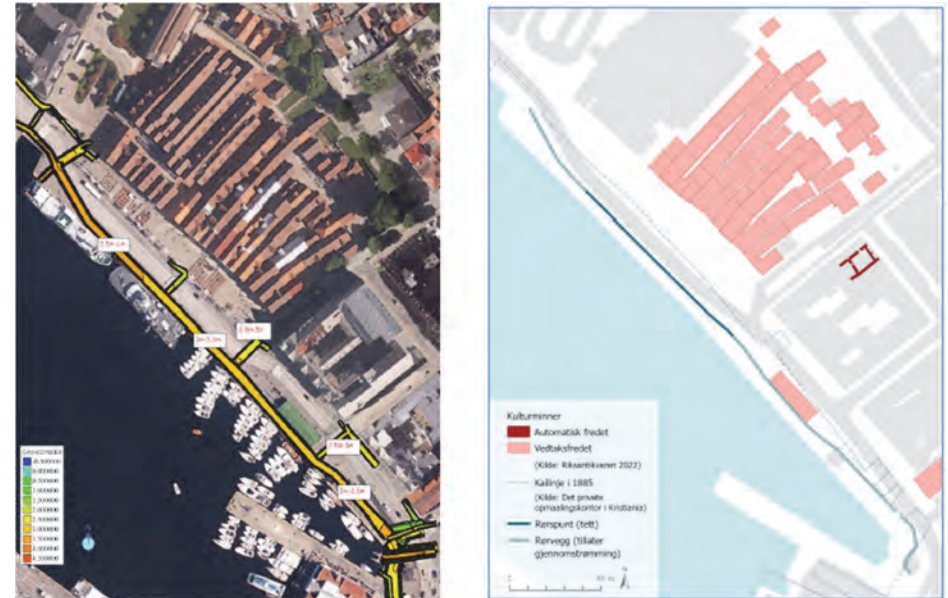
Fig. 4.19: The new ditch for infrastructure (left) and planned pile wall along Bryggen Quay (©Norconsult asplan viak)
