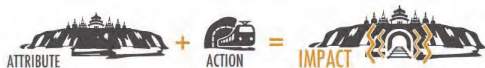
Figure 6.8. The impact on a historic urban environment created by sound and vibration from a proposed action. An impact is the interaction of the proposed action with an attribute of the World Heritage property. In this example, the vibration from a proposed action may have an impact on the buildings and weaken their structural stability. Where these buildings are an attribute of the World Heritage property, this would lead to a loss of Outstanding Universal Value.
